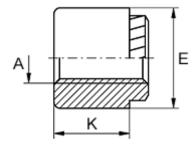
Female thread A = M2,5 Height K = 7 Hole diameter +0.1 = 4.2 Min distance to edge = 2.4 Min material thickness = 1.5 Outer diameter E = 6
